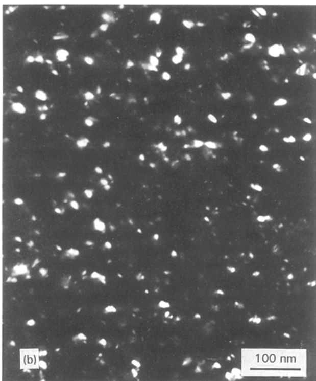
Figure 5 (a) Bright-field, (b) dark-field and (c) electron diffraction pattern of nanocrystalline nickel deposit produced at T_{on} = 2.5 ms, T_{off} = 45 ms, J_p = 1900 mA cm -2 , pH \approx 2.0 and 5 g l -1 saccharin in the bath.
